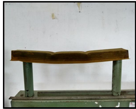
Figure5 Deflection for 1.2mm
