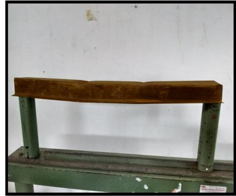
Figure6 Deflection for 1.6mm
