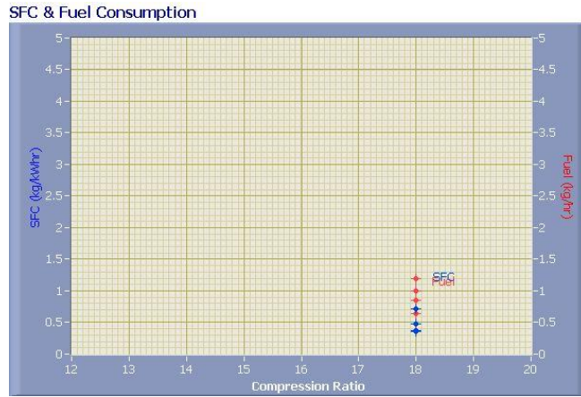
Fig.12,SFC vs CR for 10%blend with CR 18.
