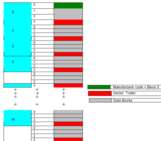
Fig 3. RFID Card Memory Structure
