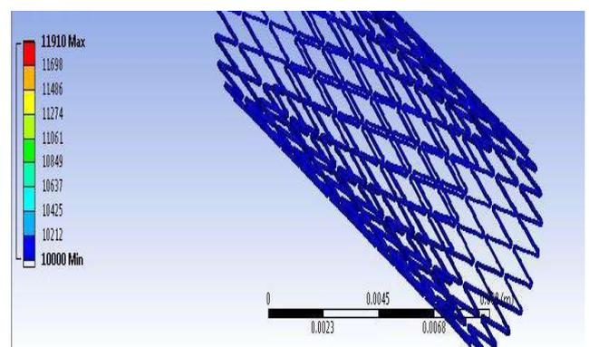
**Fig. 6 Model 2 Damage in stent of has an minimum value of 10000 cycles and a maximum value of about 11910**
