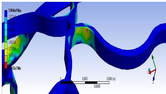
**Fig.3 Stresses are mainly distributed near the connecting bridge and on the curvature.**
