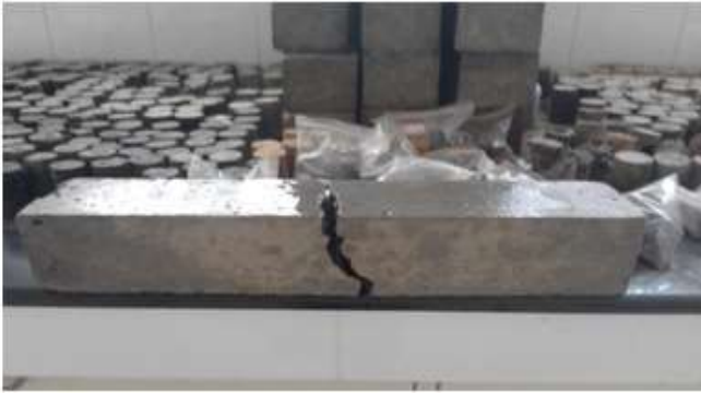
Fig 3.5 BEAM AFTER FLEXURAL FAILURE
