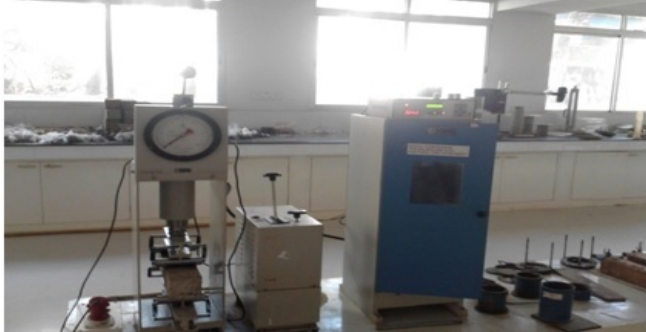
FIG 3.1 Compressive Testing Machine With Flexural Setup
