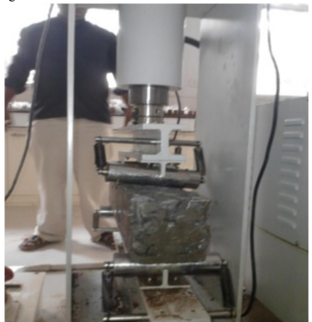
Fig 3.4 BEAM UNDER FLEXURAL LOADING
