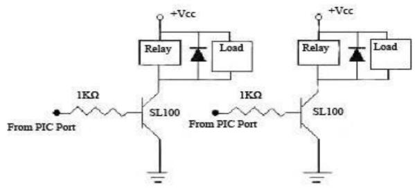
Relays are electromagnetic switches, which provide contact between two mechanical elements. Relays have a coil which works on 12V dc power supply and provides DPDT action as an output. In general relays provide potential free contacts which can be used for universal function like DC, AC voltage switching and to control bigger electrical switch gears.
