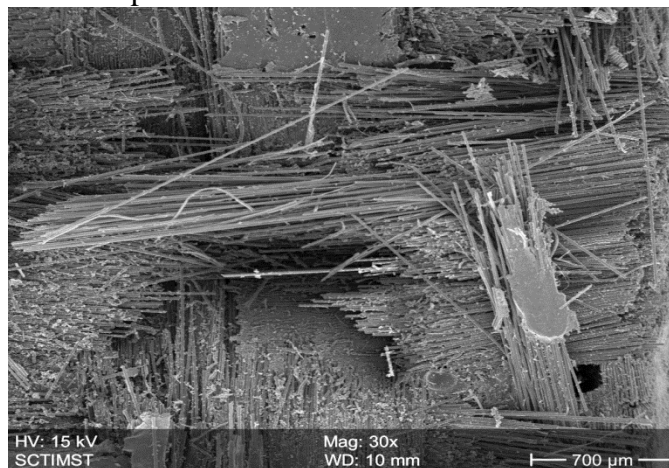
Fig.5 SEM analysis micrograph of banana fiber reinforced polyester composite subjected to tensile loading
