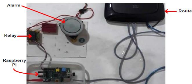
Fig. 6. Server system prototype
