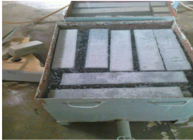
Figure 1: Test Specimens 100×100×500mm
