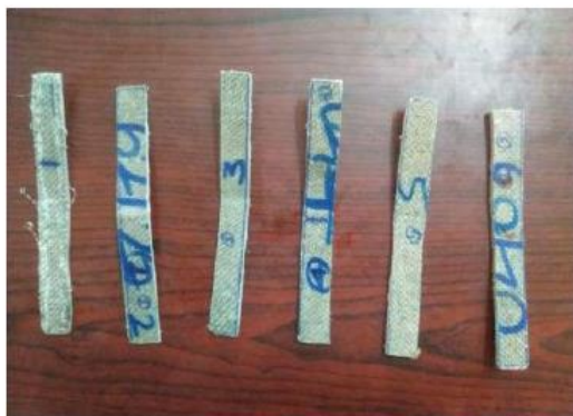
Fig – 3.3 Specimen Samples after Flexural Test
