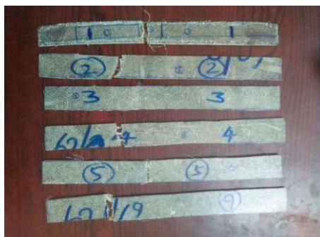
Fig – 3.1 Specimen Samples after Tensile Test
