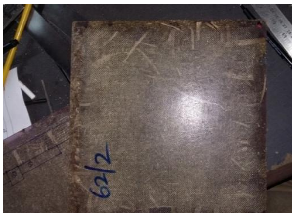
Fig 2.4 Natural Fibre Hybrid Composite Material Sheet
