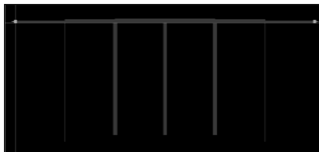
Figure 2 Layout of the Multi-band BPF Design
