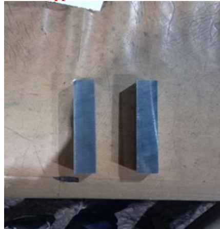
Fig 11: Specimens after Milling operation
