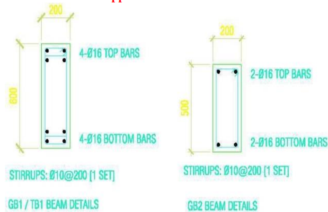
Fig 4.2 Plinth Beams
