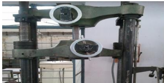
Fig 2.3 Composite Laminate on Universal Testing Machine
