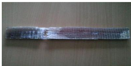
Fig 2.4 Laminate after Applying Tensile Strength
