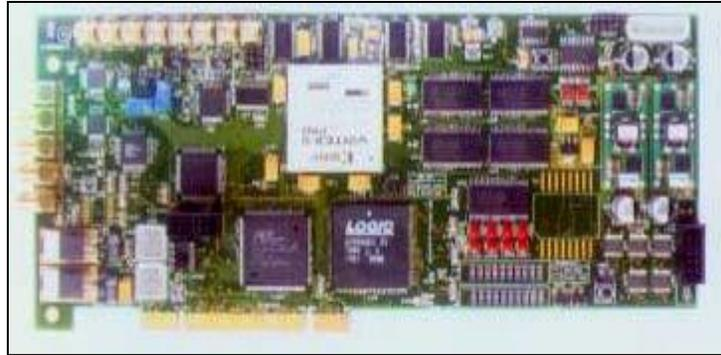
**Figure 6 High speed Image Processing Card**
