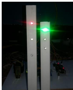
Fig. 7. Traffic Lights using LEDs
