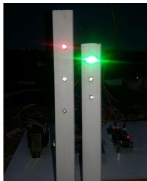
Fig. 7. Traffic Lights using LEDs
