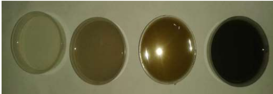
Figure 1 Films made with the help of solution cast method (a) PVP: NH 4 I+0.1wt% CNT, (b) PVP: NH 4 I+0.2wt% CNT, (c) PVP: NH 4 I+0.3wt% CNT and (d) PVP: NH 4 I+0.4wt% CNT
