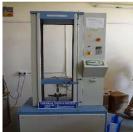
Figure 12 Universal testing machine (UTM) with three-point bending fixture
