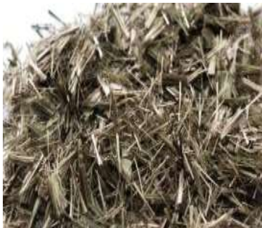
Figure 2 (a) Short basalt fiber, (b) Mat basalt fiber, (c) Continuous basalt fiber
