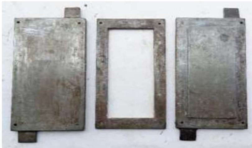
Figure 8 Open and closed part of the mold with cavity
