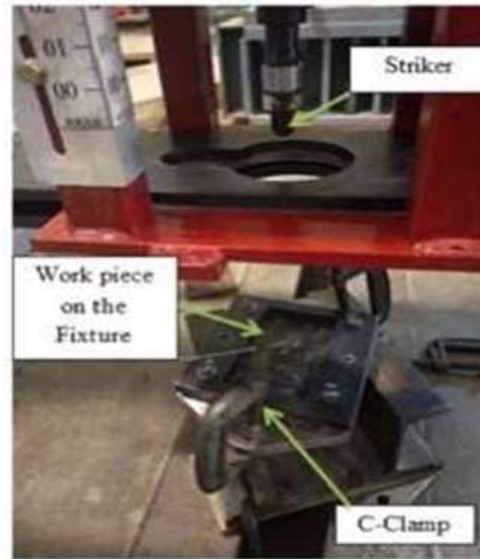
Figure 13 Low velocity impact setup
