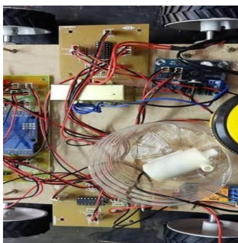
Fig 4.3: Water pump set up with 4 channel relay
