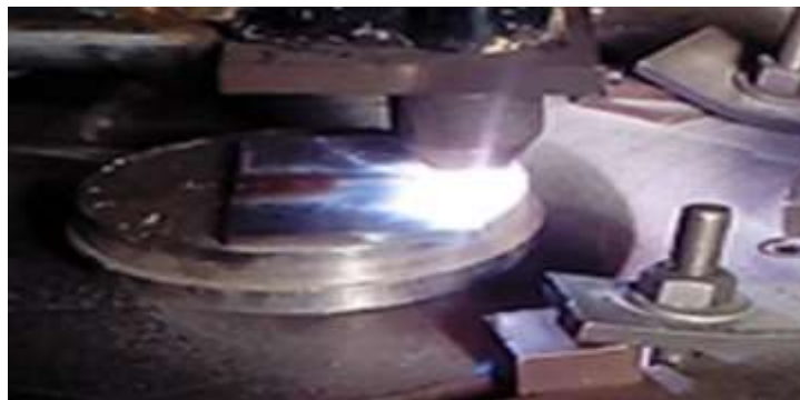
Figure 11. Stainless steel materials during welding process by plasma arc method
