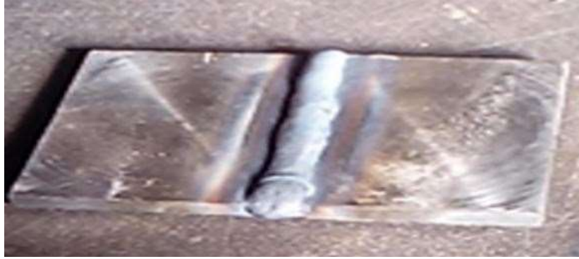
Figure 12. Stainless steel material to be tested after welding
