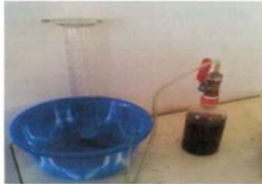
Fig : Measurement of the biogas using water displacement method
