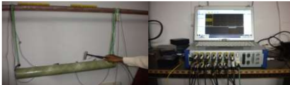
Figure 7 Vibration testing setup
