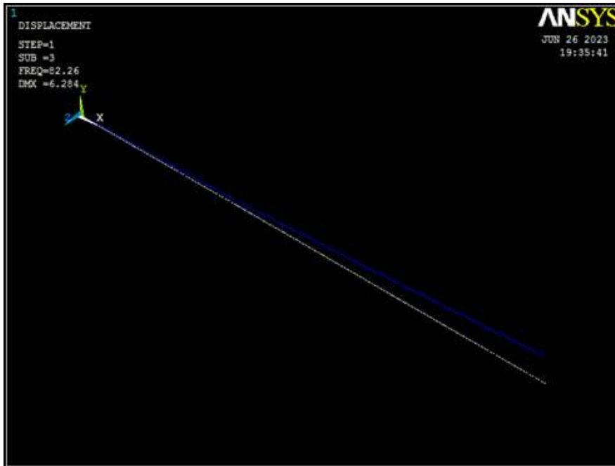
Figure 4. Third set modal solution for cantilever beam
