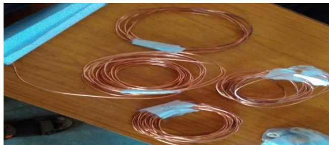
Fig. Cutting of capillary tube at variable length
