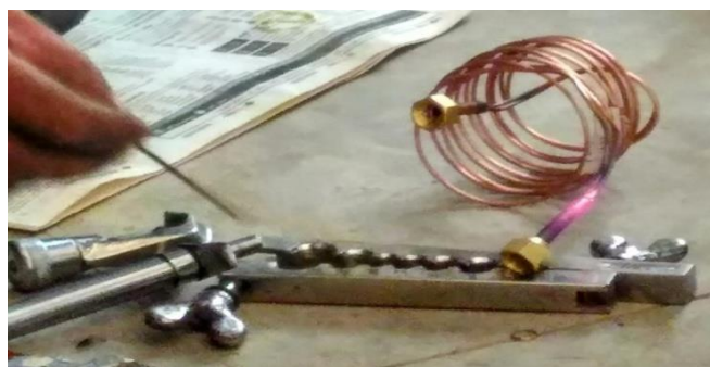
Fig. Shaping and brazing of capillary tube
