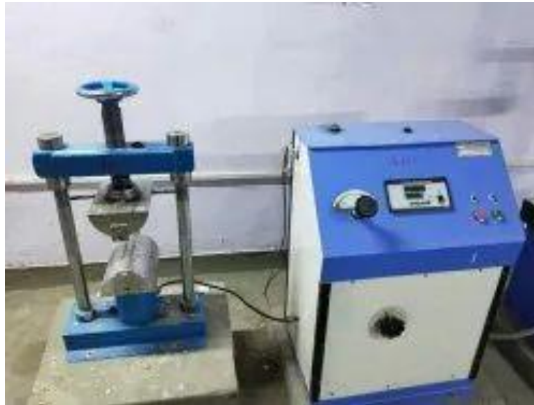
Figure 2: Machine for split tensile testing
