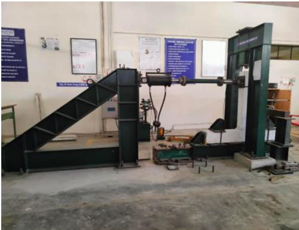
Fig. 4 Experimental setup for the beam-column joint
